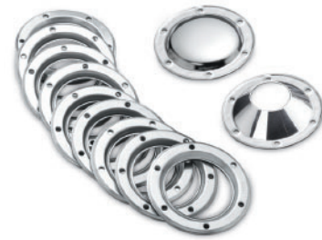
SuperTrapp tuneable discs, open and closed end caps.
