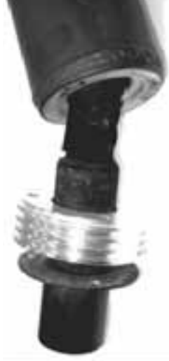
Thrust Chamber Installed correctly in muffler and ready to be bolted together.
